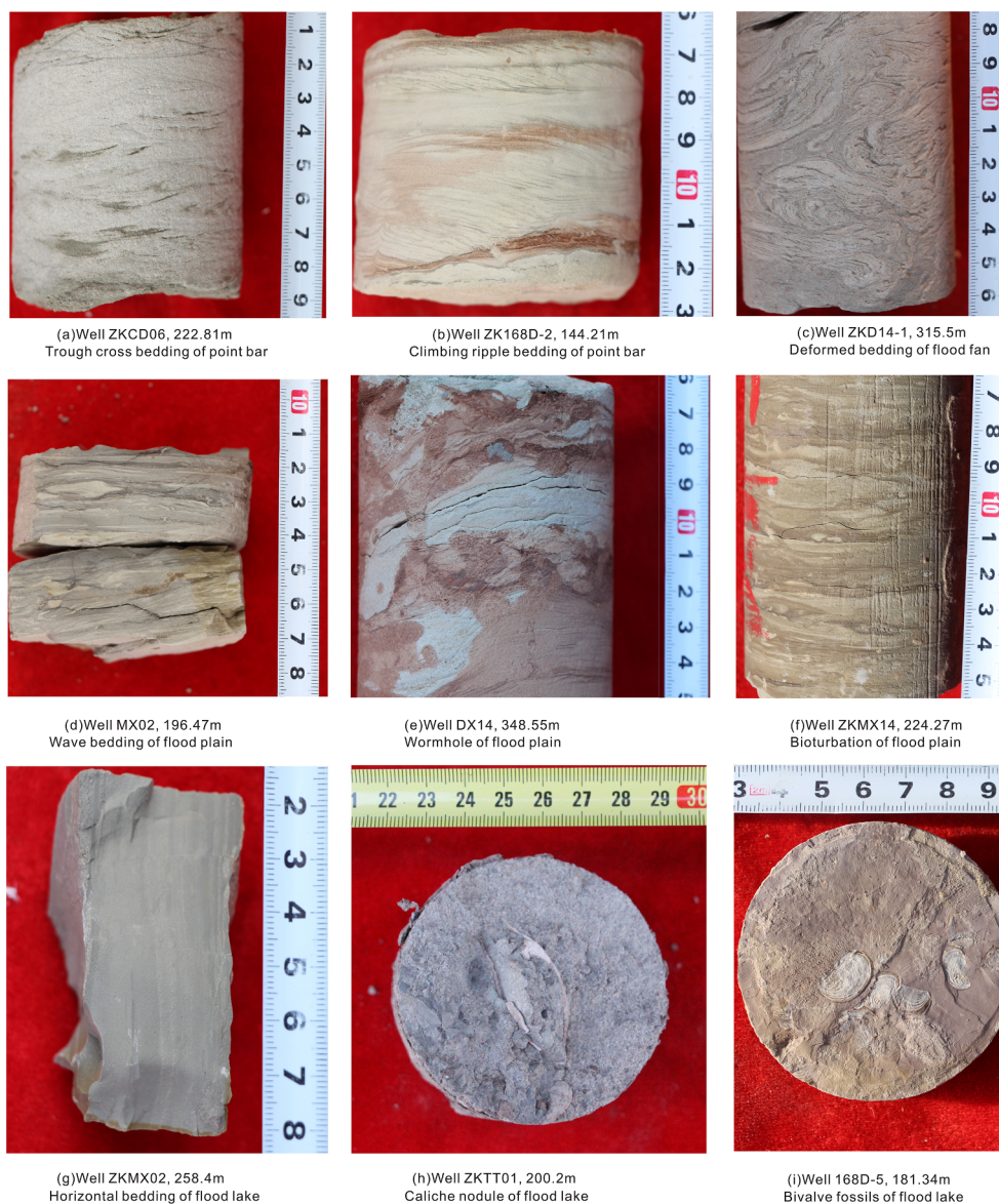
Fig. 5. Typical sedimentary structure phenomenon in core of meandering river facies.
