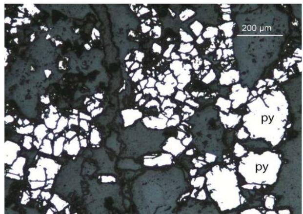
Figure 19: Hop Hoa-1. Veinlets of pyrite; reflected light, uncrossed polars.
