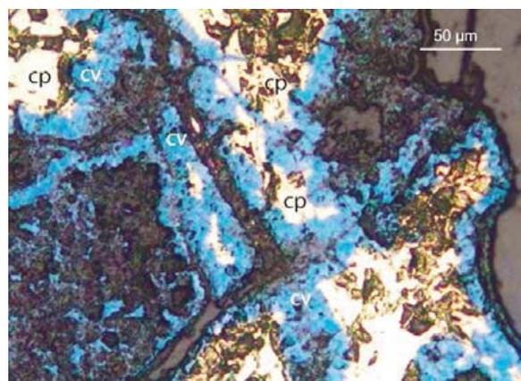
**Figure 50:** Lang Sen-1-2C. Stockwork veining of chalcopryite (cp) replaced by covellite (cv) in a matrix of brecciated quartz fragments of later stage of quartz veins after the cp; reflected light, uncrossed polars.
