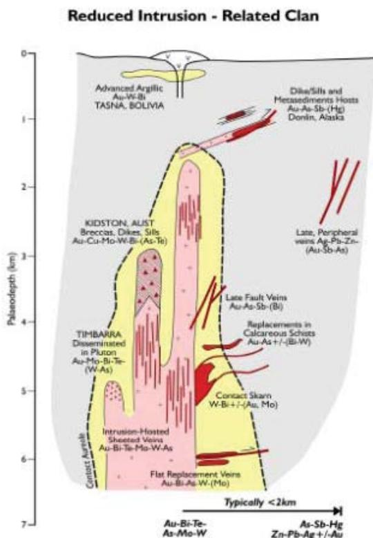
Figure 71: Typical Types of Intrusion-Related Mineralization [23].
