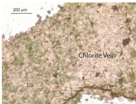
**Figure 62:** LangSen-3-4A. Chlorite vein; transmitted light, Uncrossed polars.
