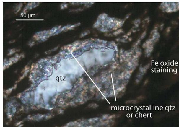
**Figure 23:** Hop Hoa-2A. Enlarged view of an augen structure showing recrystallization of microcrystalline quartz or chert inward to a single coarse grain of quartz; transmitted light, crossed polars.
