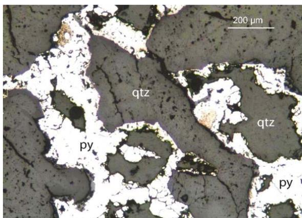
**Figure 55:** Lang Sen-2-3B-1. Irregular quartz-pyrite veining; reflected light, uncrossed polars. Small remnant, yellow mineral within pyrite (chalcopyrite or gold?).
