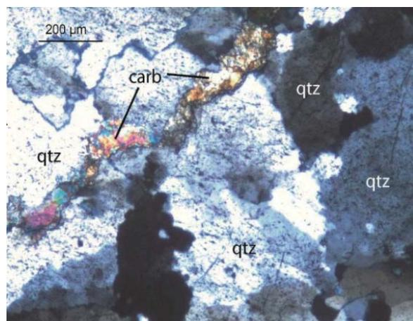
**Figure 53:** Lang Sen-2-3B-1. Silicified material cross-cut by carbonate veinlet; black mineral also quartz(at angle of extinction); scattered with very small grains of sericite in quartz; transmitted light, crossed polars.
