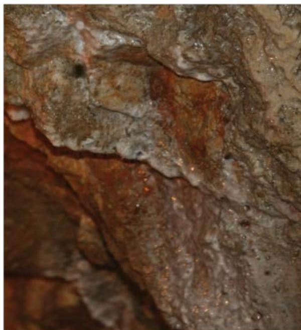
**Figure 14:** Mining Face at Hop Hoa Mine. Note Pyrite Reflections.
