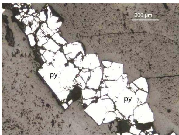
**Figure 38:** Vai Dao-3. Pyrite veinlet in quartz (gray) with disseminated fine-grained sericite (a phyllosilicate): reflected light, uncrossed polars.
