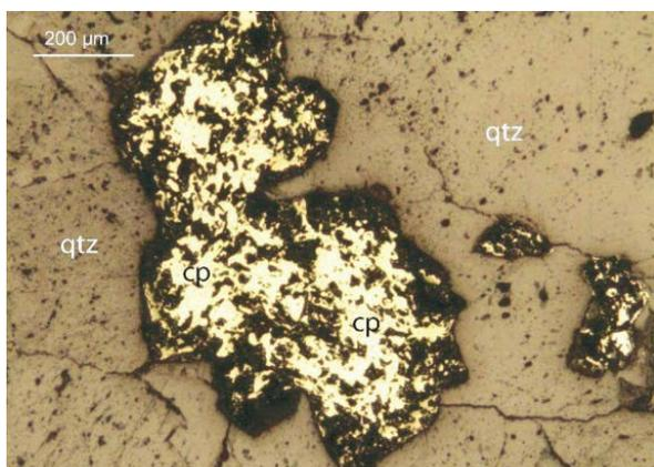
**Figure 56:** Lang Sen-2-3B-1. Disseminated chalcopyrite (cp) in quartz; reflected light, uncrossed polars.
