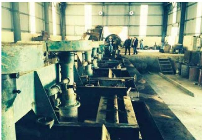
**Figure 78:** Flotation Cells at the Processing Plant.
