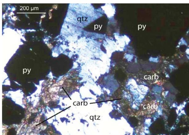
**Figure 34:** Vai Dao-1. Vein containing pyrite-quartz-carbonate; transmitted light, crossed polars.
