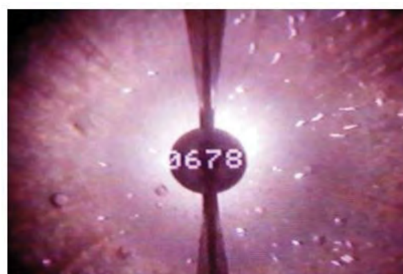
Figure 28: Minor Natural Gas Bubbles Rising in MUD Well Casing at Depth 678 Feet. (From [10])
