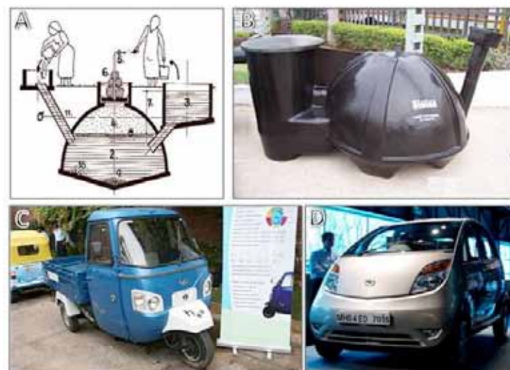
Figure 30. The 'flow chart' of a family-sized Indian biogas generator (A) and its modernised commercial version (B). Hydrogen-powered three-wheeled utility vehicle (C) and the similarly hydrogen-propelled Indian 'people's car' (D).
