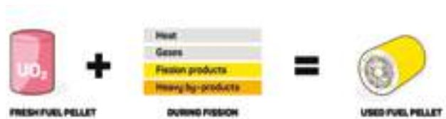
Figure 5.7: The chemical make-up of used fuel
