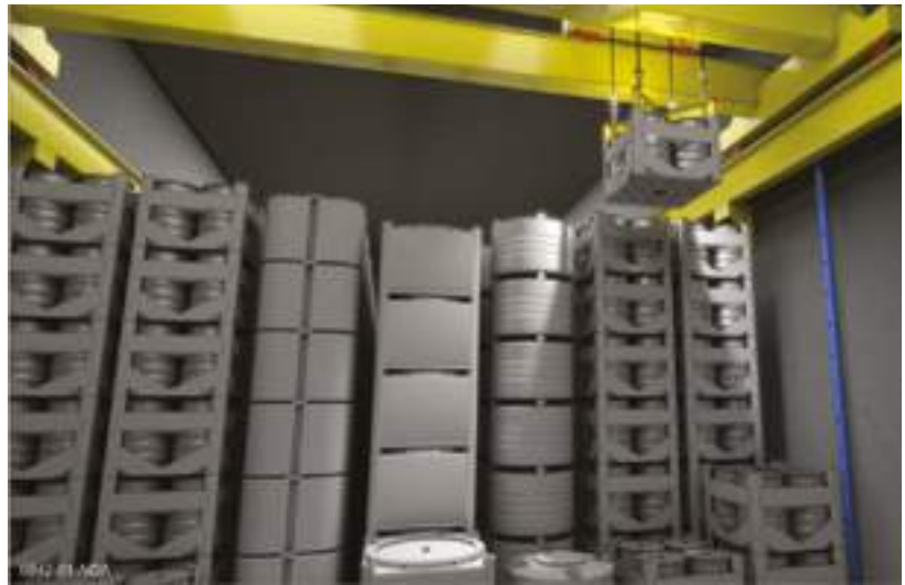
Figure 5.15: Schematic illustration of a medium-depth ILW disposal facility, with artist's rendering of a disposal vault with overhead crane for ILW disposal
