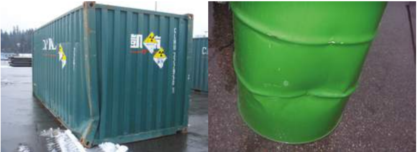
Figure 9.1: Damage to UOC shipping and packaging containers
