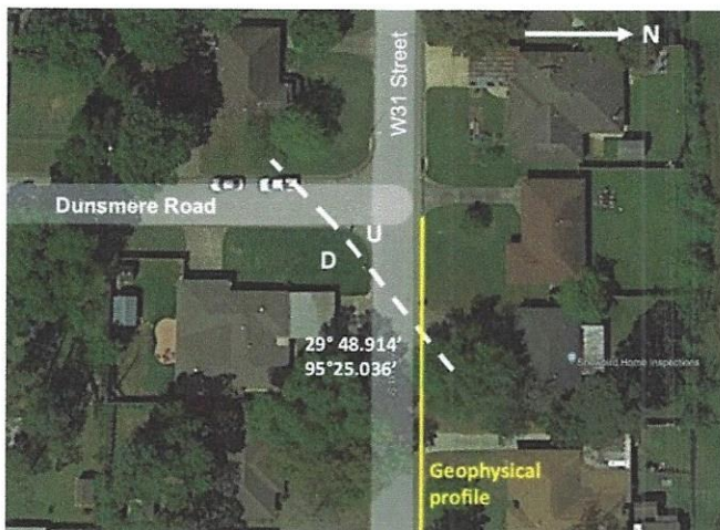
Figure 8. Site map showing the approximate location of the Eureka fault crossing West 31st Street and Dunsmere Road. Fault deformation is highly visible on the asphaltic pavement of West 31 Street. The yellow line indicates the location of geophysical profiles.
