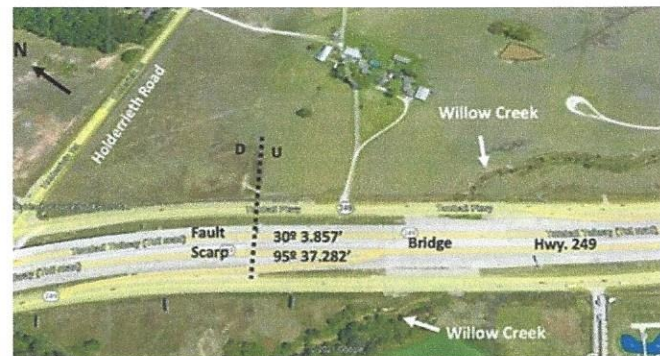
Figure 19. Site map showing the location of Willow Creek fault, which is located between Willow Creek and Holderrieth Road. Note that willow Creek makes a sharp turn across the interpreted fault location. There were also asphalt patches to the South of the Creek and on the bridge. It is interesting to note that the farmland to the northeast (where the farmhouse is located) is undeveloped.
